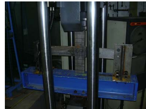
Load bearing capacity testing on welded joints
