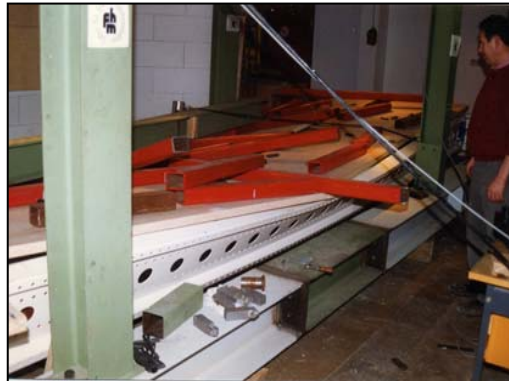
Load bearing capacity test on \Sigma - Profiles
