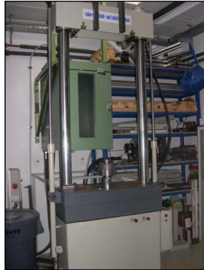
testing machine with acclimating chamber (-20 to 90°C)
