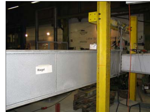
Full scale testing of traffic sign bridges
