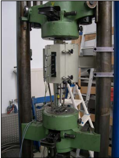
1000 kN testing machine with inductive heating oven (Tmax = 900°C)
