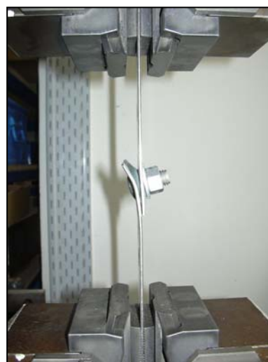
Ultimate load test on mechanical connections
