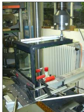
Fatigue test on silicon bonded panels
