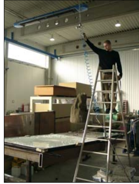
Testing of accessible glass according to GS Bau 18
