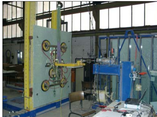
Dynamic post breakage behaviour of vertical glazing systems
