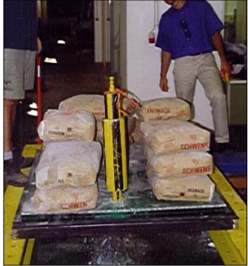
Testing of walkable glass
