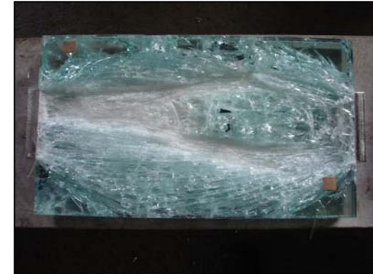
Test serial of connecting detail of glass stairway
