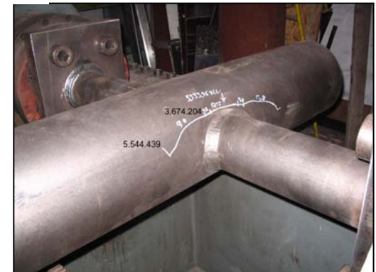
Fatigue test on thick walled hollow sections "scale effect"
